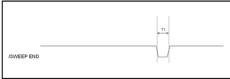
Figure C-3 Pulse width of /SWEEP END
